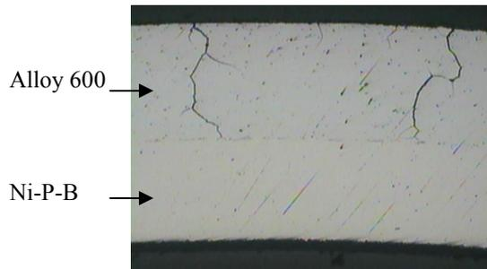
Fig. 2. Optical micrograph examined after C-ring test for Ni-P-B electrodeposit. C-ring test was carried out by applying 180mV above an open circuit potential in 40wt% NaOH solution at 315°C for 7 days.
