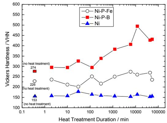
Fig. 3. Vickers hardness value for Ni, Ni-P-Fe and Ni-P-B electrodeposits as a function of heat treatment duration at 343°C.
