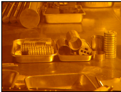
Figure 4. Cutting and dismantling the thermal media with an outer pipe.
