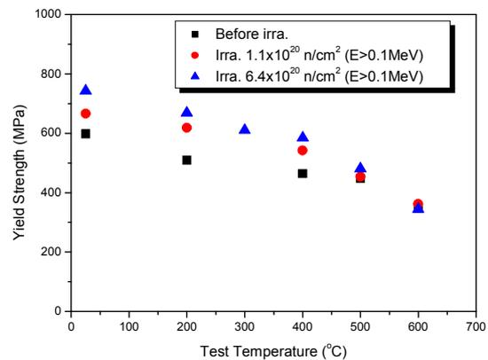
Fig. 1. Change of yield strength with neutron fluence
