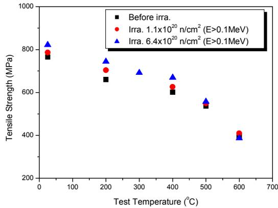
Fig. 2. Change of tensile strength with neutron fluence
