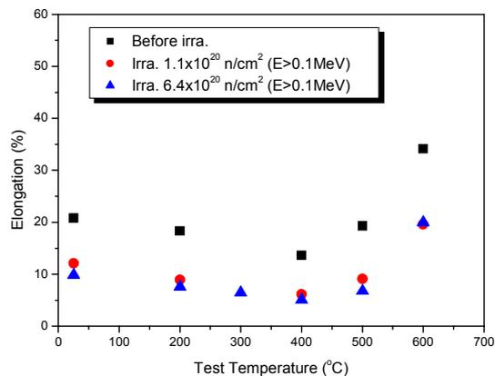
Fig. 3. Change of elongation with neutron fluence
