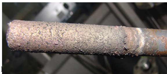
electrorefining of uranium (500 °C, UCl 3 : 9wt%, current density : 130mA/cm 2 for 3 hrs).
