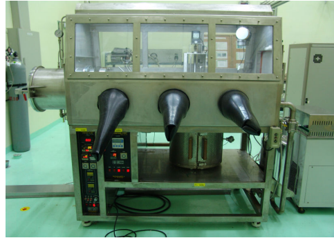
Fig. 1. Glove box for the uranium electrorefining.
