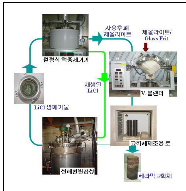
Figure 1. Salt-loaded ceramic waste form fabrication procedure
