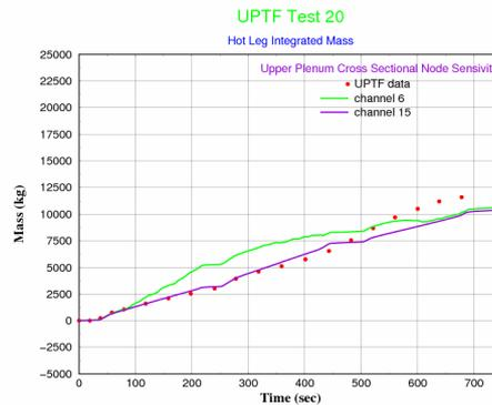
Figure 5. Integrated Hot Leg Mass Flow Rate
