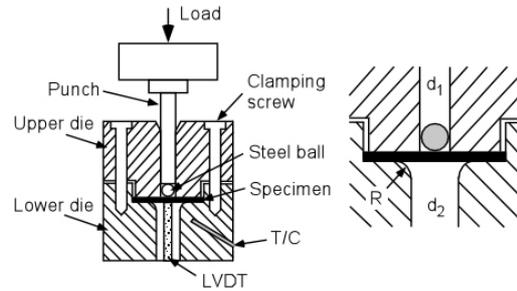
Figure 1. Schematic drawing of SP test.
