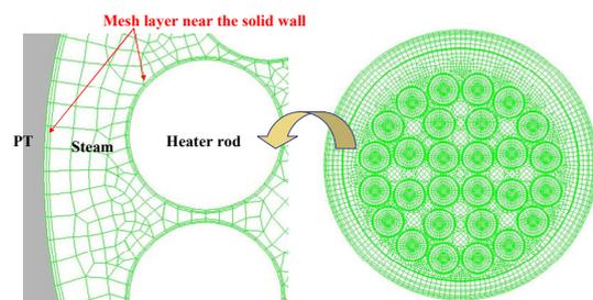
Figure 2 Mesh generation of the CS28-2 test section
