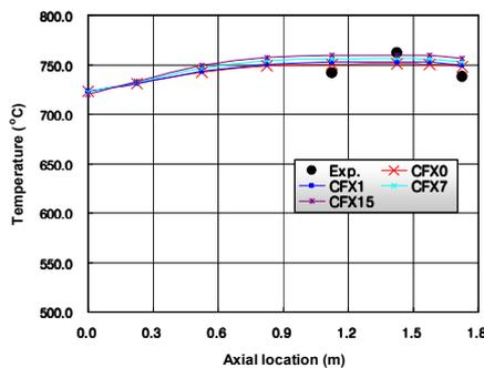
Figure 4 Axial temperature profile for the middle ring
