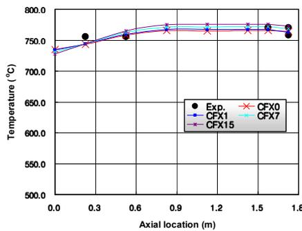
Figure 3 Axial temperature profile for the inner ring
