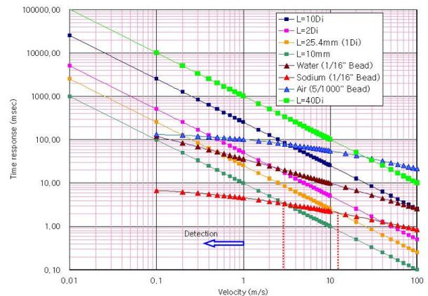
Figure 2. Time response of the thermocouple with velocity
