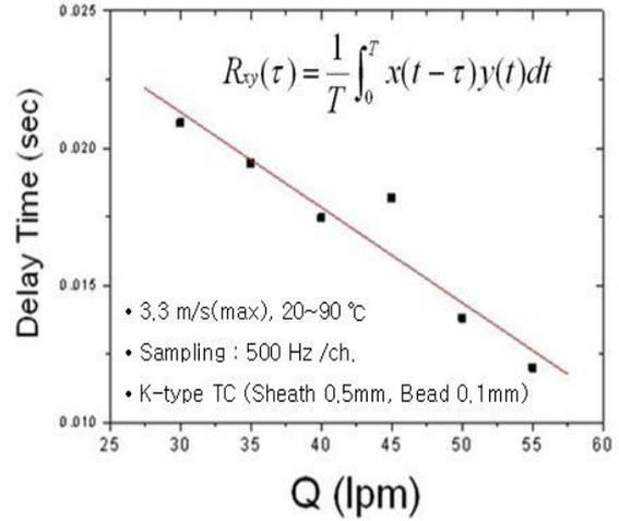
Figure 4. Calculated delay time with water velocity
