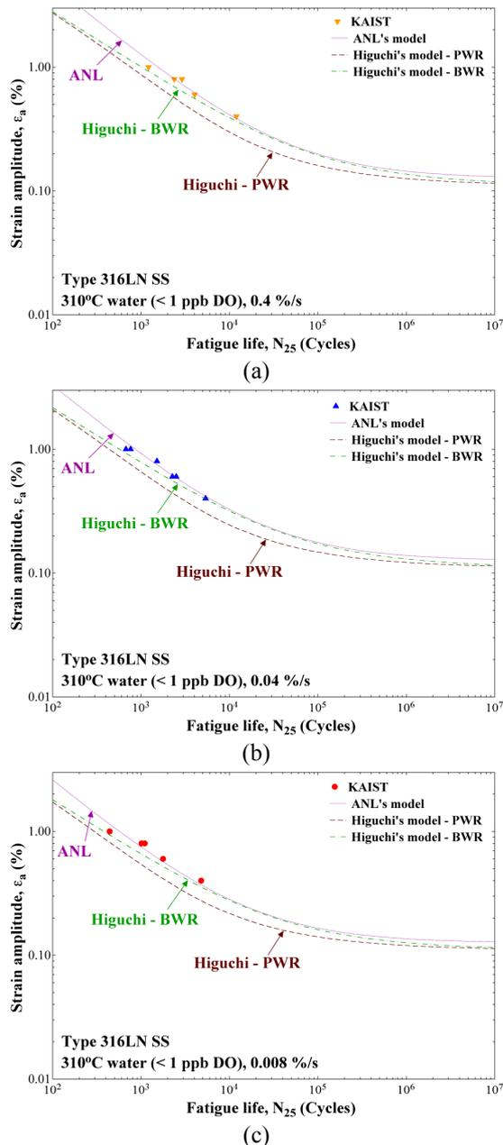
Figure 2. Comparison of the fatigue lives generated in this study and other researchers' models: (a) 0.4, (b) 0.04, and (c) 0.008 %/s.
