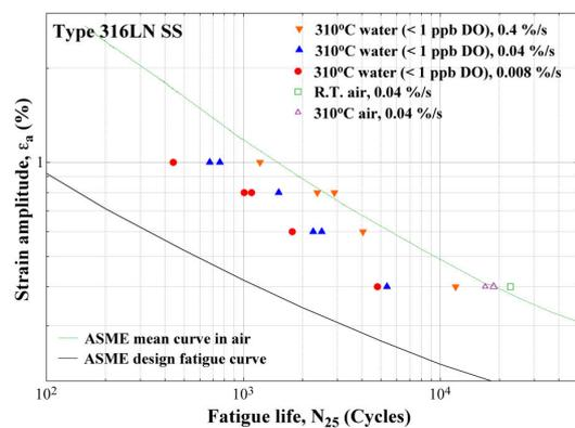
Figure 1. Fatigue lives of type 316LN SS with various strain rates in air and 310°C low oxygen-containing water.
