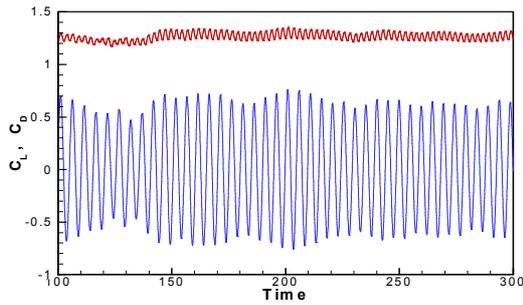
Fig. 2 Time-histories of the drag and lift coefficients for the circular cylinder at  $Re=300$
