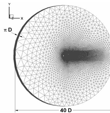
Fig. 1 Solution domain and mesh for a 3-D cylinder flow
