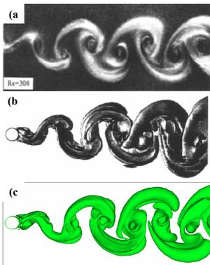
Fig. 4 Vortical flow behind the cylinder, (a) experimental visualization by using aluminum flakes (Williamson), (b) DNS result by Noack, (c) current numerical result
