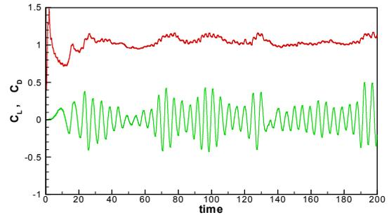
Fig. 5 Time-histories of the drag and lift coefficients for the circular cylinder at  $Re=3,900$
