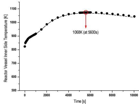
Figure 1. Maximum temperature of reactor vessel inner wall
