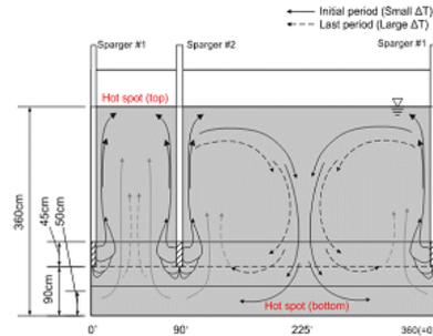
Figure 6. Assumption of natural convection pattern in IRWST
