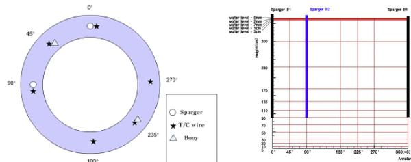
Figure 2. Location of Thermocouples
