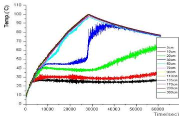
Figure 4. Temperature transient (Initial water level : 3.6m, place : 0°)
