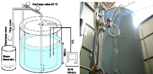
Figure 1. Schematic diagram and picture of the experimental facility
