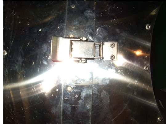
Fig. 1 Buckle Fastener Type Insulator configuration
