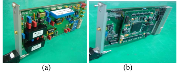
Figure 2. The picture of (a) Signal conditioning module(SCM), (b) Data acquisition module(DAM)
