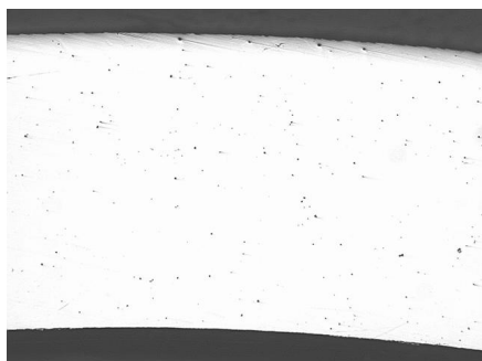
Figure 3. The microstructure of tube expanding transition region, under abnormal explosive expansion, after 4000 hour duration under 40%NaOH, 300°C.
