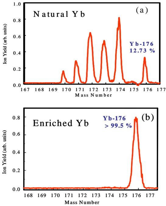
Fig. 3. Time of flight mass spectrum (a) natural Yb (b) after the selective photoionization.
