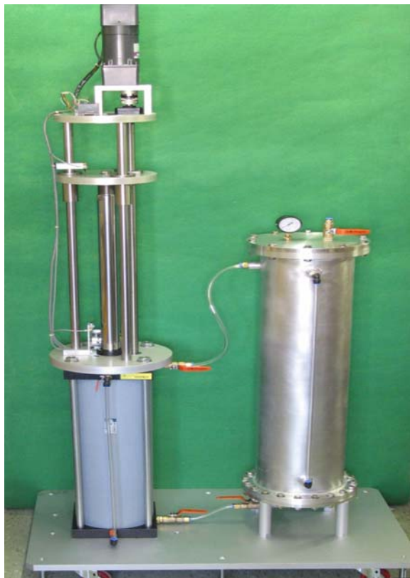
Figure 3. Fabricated test pot of the cylinder type stub
