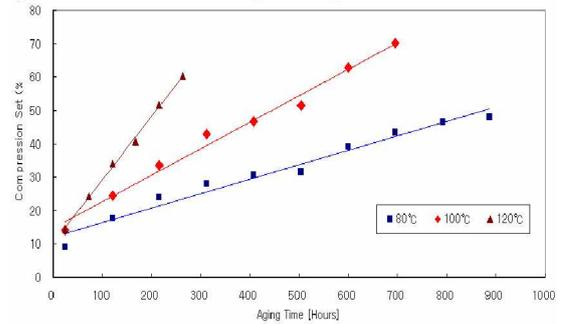
Figure 1. Compression Set for NBR O-ring
