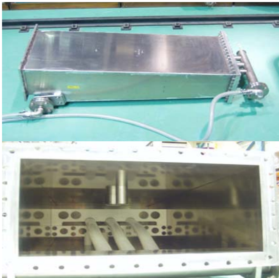
Figure 1. external and internal shapes of manufactured 100kW magic tee dummy load.
