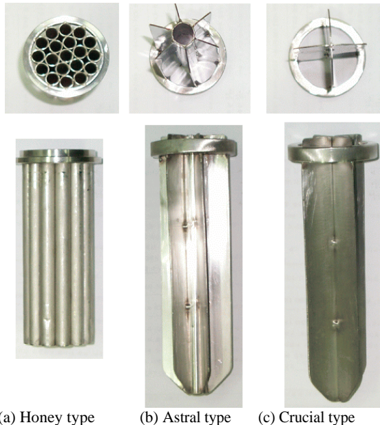
Figure 1 Shapes of flow straighteners
