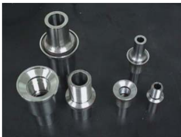
Figure 1. Prepared Dissimilar Metal Joint Specimens for brazing
