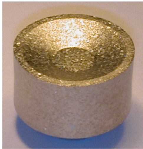
Fig. 3. Zr-U alloy sintered at 1500°C in high vacuum for 2 hours.
