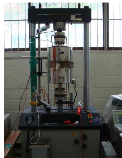
Fig. 2 High temperature FCG test facility
