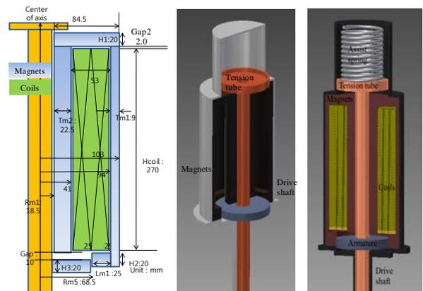
Fig.3 An update design concept of electromagnet core
