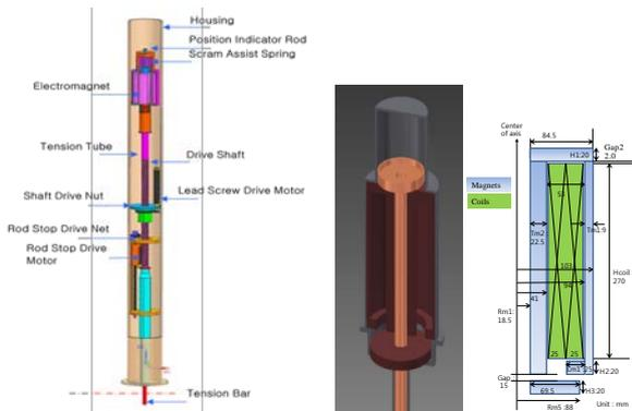
Fig.1 Initial concept of electromagnetic device
