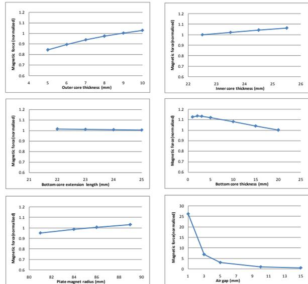
Fig. 2 Electromagnet forces between electromagnet and armature (drive shaft and tension tube)
