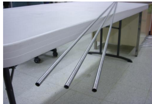
Fig. 1 Fabrication of preliminary HT9 cladding tube
