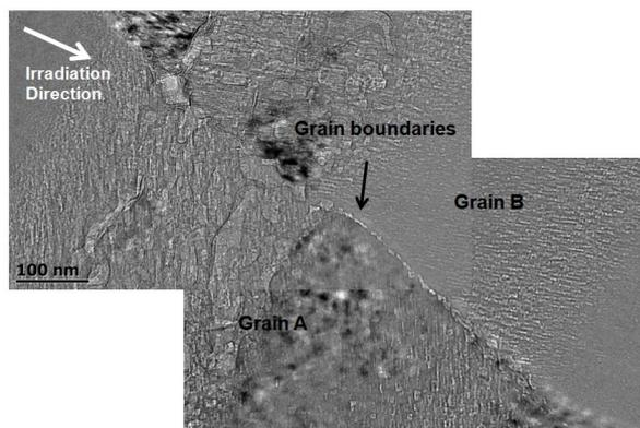
Fig. 2. Cross-section image of proton irradiated (120 keV,  $2.0 \times 10^{18}$  ions/cm<sup>2</sup>) beryllium, observed by TEM. Two different grains (Grain A and B) are irradiated simultaneously. The distribution of vacancies was affected by the crystal orientation and grain boundaries.
