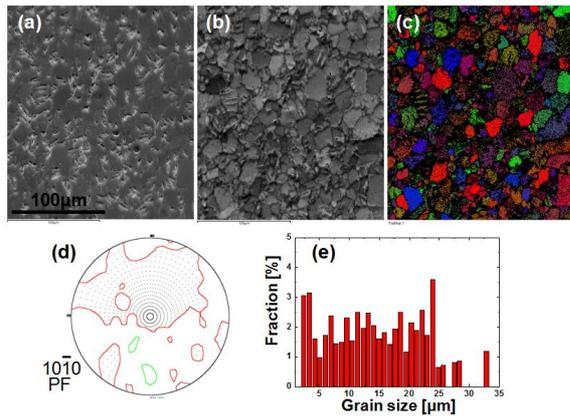
Fig. 1. Microstructure of a beryllium reflector block (S-200-F). The grain shapes are shown through a (a) SEM image of the etched surface, (b) the EBSD band contrast, and (c) a crystal orientation map, respectively. A corresponding (d)  $10\bar{1}0$  polefigure and (e) the grain size distributions are shown.
