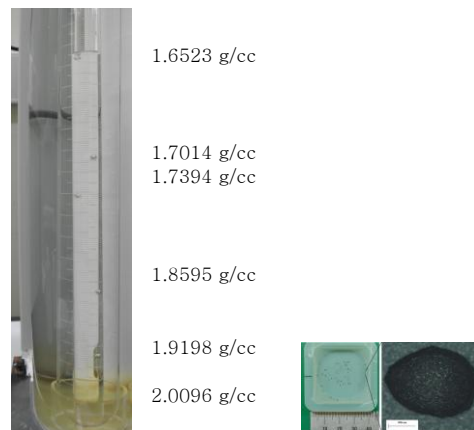
Fig. 2. Density gradient column for density measurement of O-PyC coating layers.
