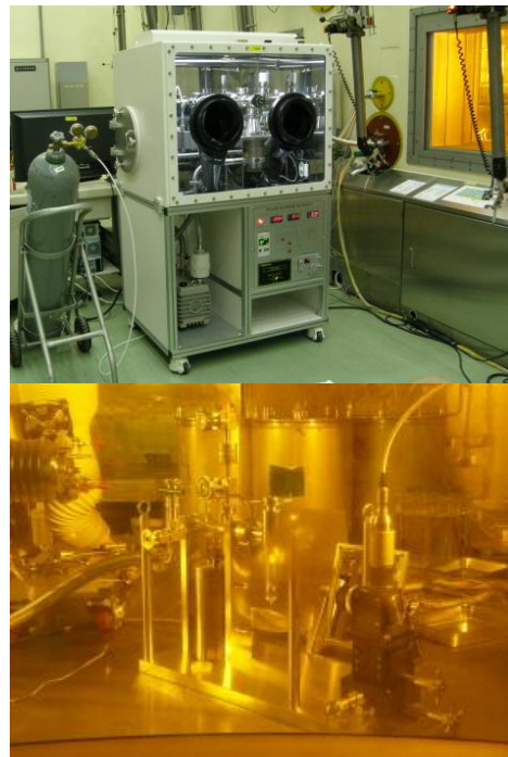
Fig. 1 Laser puncturing system in IMEF
