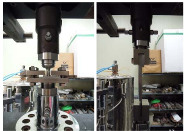
Fig. 5 Test photograph of the welding joints by tensile test.
