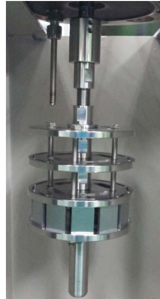
Fig. 2. Feature of the test specimen holder.
