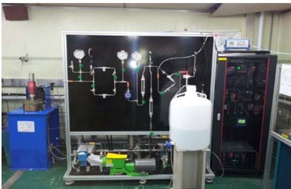
Fig. 1. Photograph of FAC evaluation test loop.
