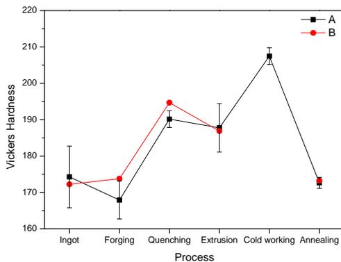
Fig. 3. Changes in hardness of HANA-4 tube shells with the manufacturing process
