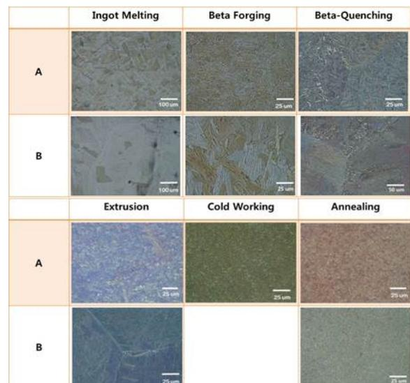
Fig. 1. Microstructures of HANA-4 tube shells different with manufacturing process between two manufacturers.
