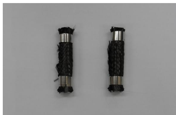
Fig. 2. Model samples of the metal-ceramic hybrid cladding tube, used for impregnation
