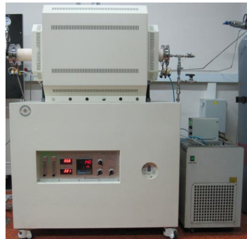
Figure 3. Apparatus (tube furnace) for high temperature oxidation of coated Zr alloys in steam
