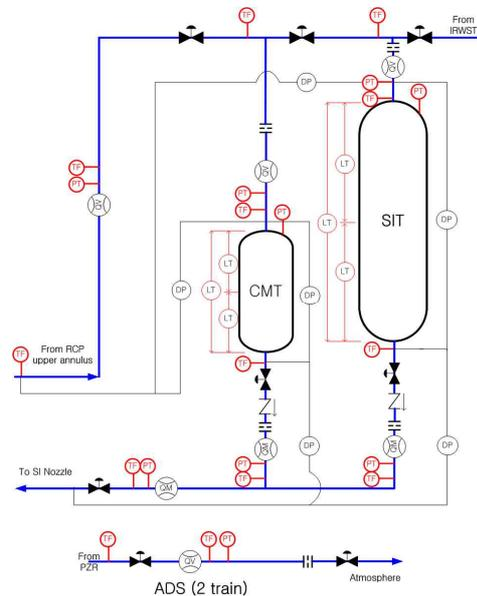
Fig. 2 Schematics of the test facility for SMART passive safety system
