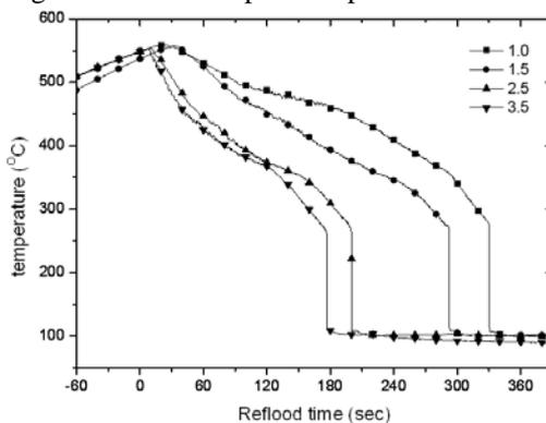
Fig. 6 Transient temperature profiles at 950mm
