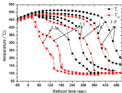
Fig. 4 Transient temperature profiles at 803mm
