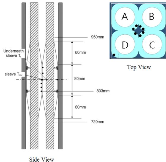
Fig. 2 Configuration of the blockage simulator
