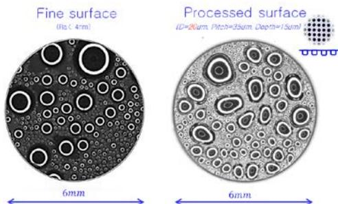
Fig. 2 Comparison of Processed Surface to Fine Surface (Visualization)
