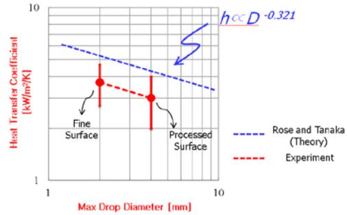
Fig. 3 Comparison of Processed Surface to Fine Surface (Heat Transfer Coefficient)
