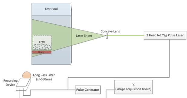
Fig. 1. Schematic Diagram of PIV/PLIF measurement.
