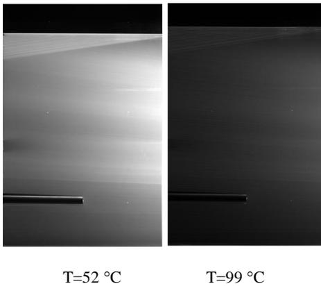
Fig. 3. LIF calibration image with different pool temperature
