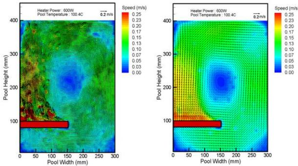
Fig. 2. Instantaneous and mean velocity vector field (Pool temperature is 100.4 °C).
