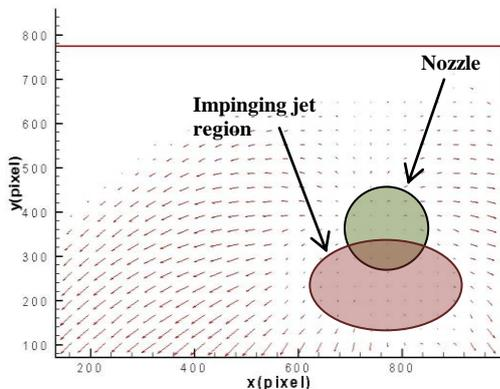
(b) Local film velocity in impingement region after PIV post-processing
