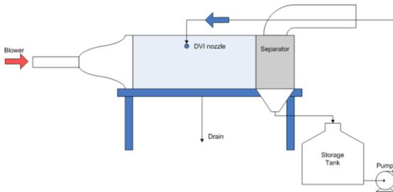
Fig. 1. Schematic view of liquid film experimental facility
