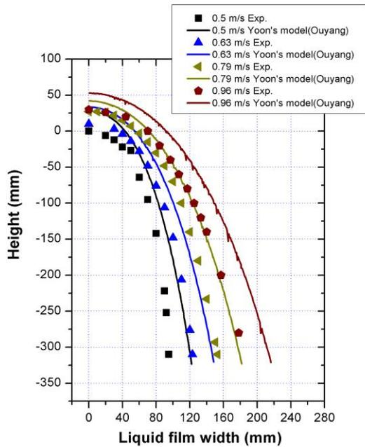
Fig. 4. Assessment result of Yoon's model (Ouyang's wall friction model) with experimental data.
