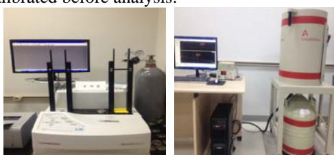
Fig.1. Low Background system and HPGe detector
