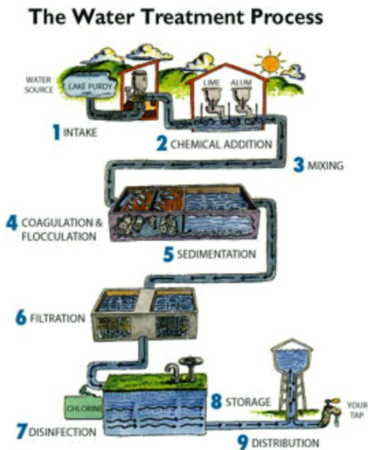
Fig. 2 Tap water manufacturing procedure (By Google image search)
