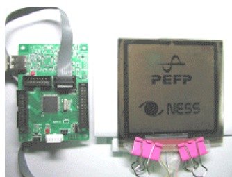
Fig. 2. LCD pilot product by using ion beam alignment process
