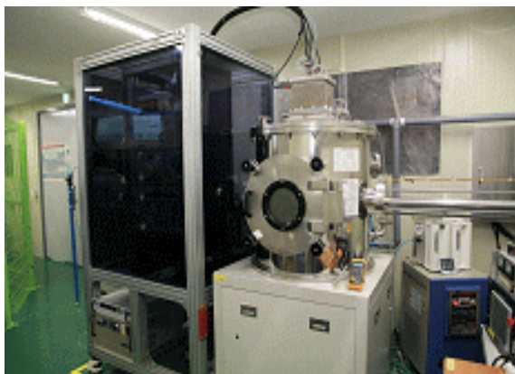
Fig1. Ion beam sputter deposition equipment.
