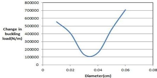
Fig. 2. Irregular Change in magnitude in buckling load following the change in hole-diameter.
