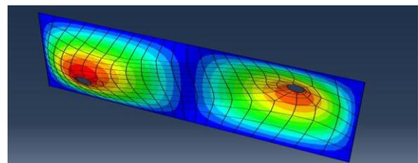
Fig. 1. Mode 1 of deformed plate
