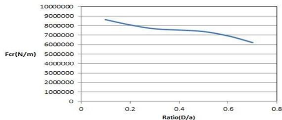
Fig. 3. Critical load versus dimension ratio ( $D/a$ )
