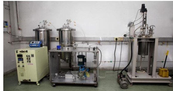
Fig. 1. Photograph of the simulated primary water test loop.
