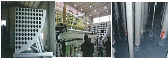
Fig. 4. Mock-up for calandria inspection
