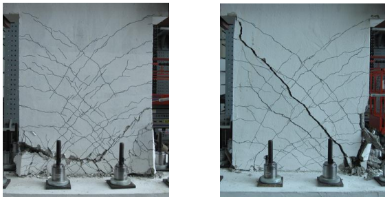
(a) SFRC specimen at 3.5% drift (b) RC specimen at 2.5% drift
