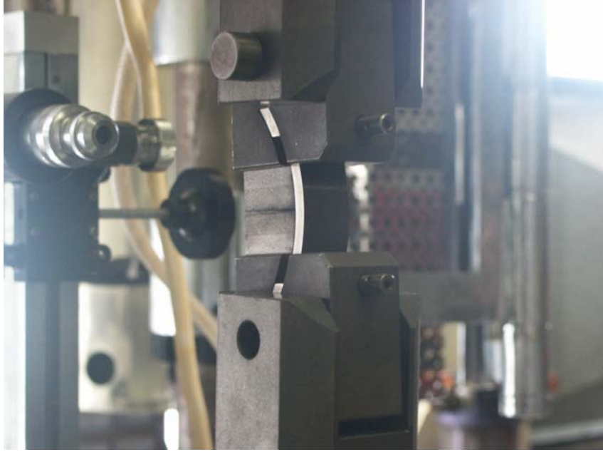
Figure 2. Curved center cracked tension specimen and specimen-fixture assembly.
