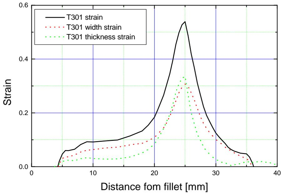
Fig. 3. Strain distribution of width and thickness along the length of the broken specimen at RT in 30° tilt tensile specimen from the transverse direction (black line, red dotted line, and green dotted line denote the total strain, the strain in width and in thickness, respectively.)
