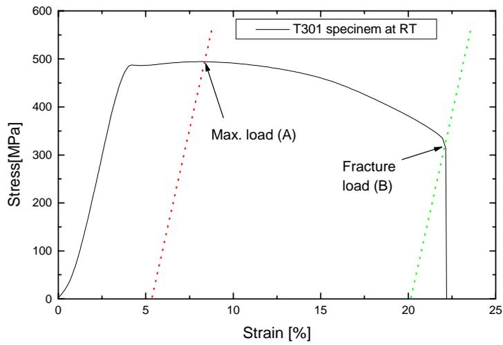
Fig. 5. Engineering strain-stress curve in the 30°-tilt specimen from the transverse direction at RT.
