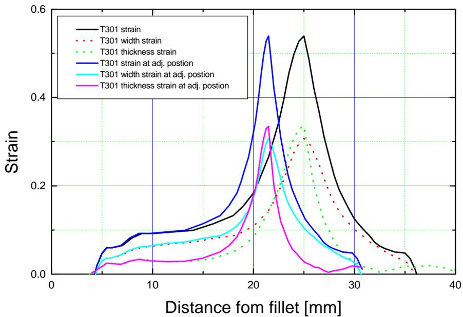
Fig. 4. Strain distribution of width and thickness along the length of the broken specimen at RT in 30° tilt tensile specimen from the transverse direction (blue line, cyan line, and magenta line denote the total strain, the strain in width and in thickness, respectively.)
