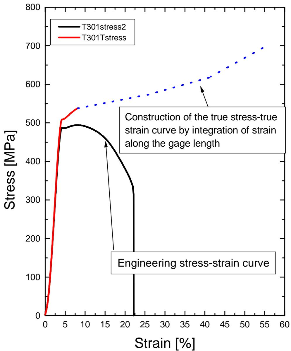
Fig. 7. True strain-true stress curve for the 30°-tilt tensile specimen from the transverse direction at RT.
