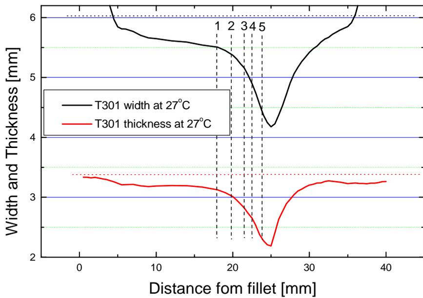
Fig. 2. Width and thickness variation along the length of the broken specimen at RT in 30° tilt tensile specimen from the transverse direction
