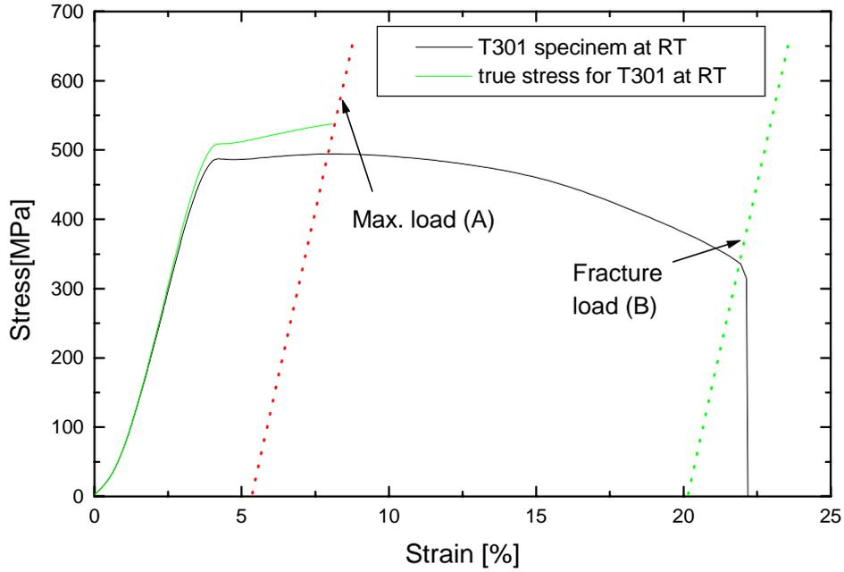
Fig. 1. Engineering and True strain-stress curves in 30° tilt tensile specimen from the transverse direction at RT.
