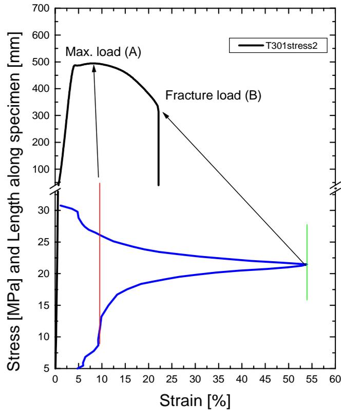
Fig. 6. Schematic illustration of the relationship between the strain in the strain stress curve and the accumulation of the strain along the gage length of the tensile specimen.
