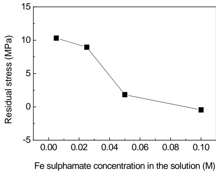
Fig. 2 Residual stresses of Ni-P-Fe alloy deposits as a function of Fe sulphamate concentration in the sulphamate bath of 1.39M Ni + 0.018M P under the condition of 50°C, pH 1 and 15A/dm<sup>2</sup>.
