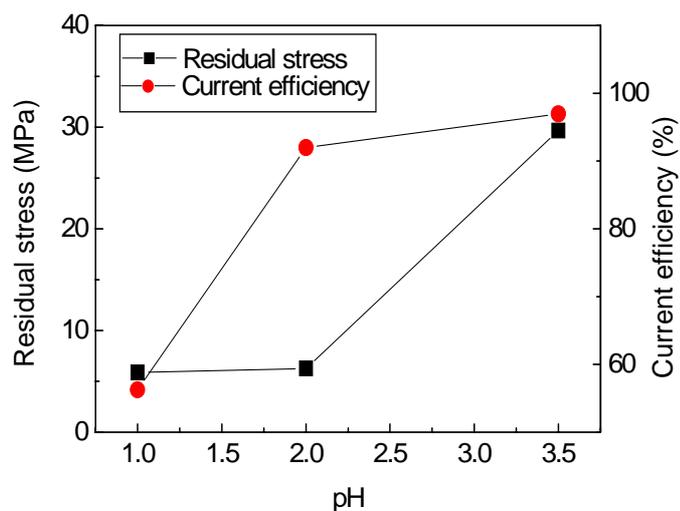
Fig. 4 Residual stresses of Ni-P-Fe alloy deposits with the pHs in the electrolytes of 1.39M Ni + 0.007M P + 0.005M Fe under the condition of 60°C and 5A/dm<sup>2</sup>.
