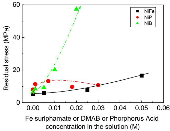
Fig. 1 Residual stresses of Ni binary alloy deposits with the concentration of various alloying element such as Fe, P and B in the sulphamate bath of 1.39M Ni under the condition of 50°C, pH 1 and 15A/dm<sup>2</sup>.
