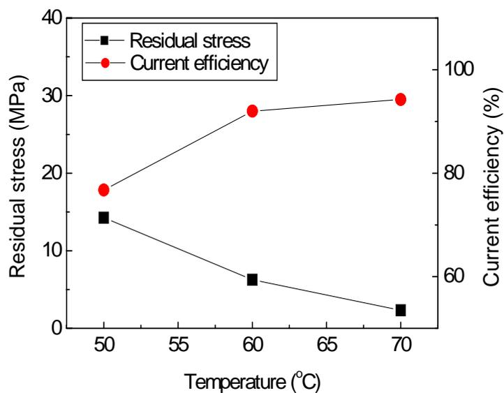
Fig. 5 Residual stresses of Ni-P-Fe alloy deposits with temperature in the electrolytes of 1.39M Ni + 0.007M P + 0.005M Fe under the condition of pH 2 and 5A/dm<sup>2</sup>.
