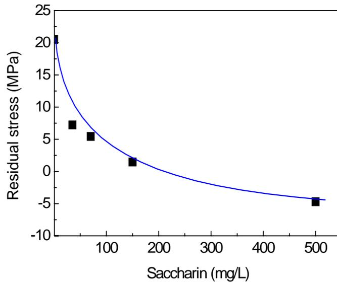
Fig. 3 Stress values measured for Ni-P-B alloy electrodeposits prepared from the baths containing various saccharin concentrations.
