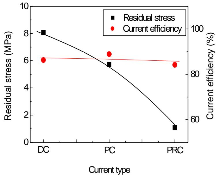
Fig. 6 Residual stresses of Ni-P-Fe deposits with current types at an average current density of  $10\text{A/dm}^2$  in the electrolytes of  $1.39\text{M Ni} + 0.007\text{M P} + 0.005\text{M Fe}$  containing various additives of saccharin, coumarin, sodiumlaruylsulfate under the condition of  $60^\circ\text{C}$  and  $\text{pH } 2$ .
